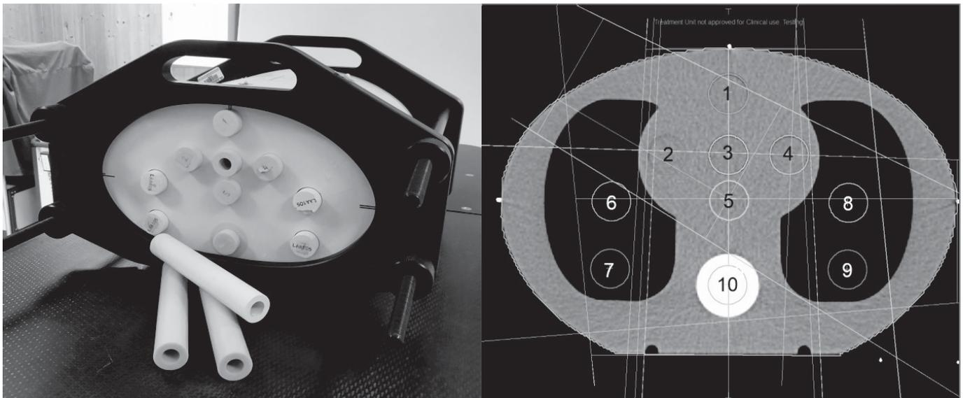
**FIGURE 1.** Photo of the semi-anthropomorphic CIRS Thorax phantom with interchangeable rod inserts (left) and its CT image (right). Positions of 10 interchangeable rod inserts are marked with numbers from 1 to 10. Five measuring points are in the water equivalent part of the phantom (grey area), four points are in the lung density equivalent material (black area), and one point is in the bone density equivalent part of the phantom.
