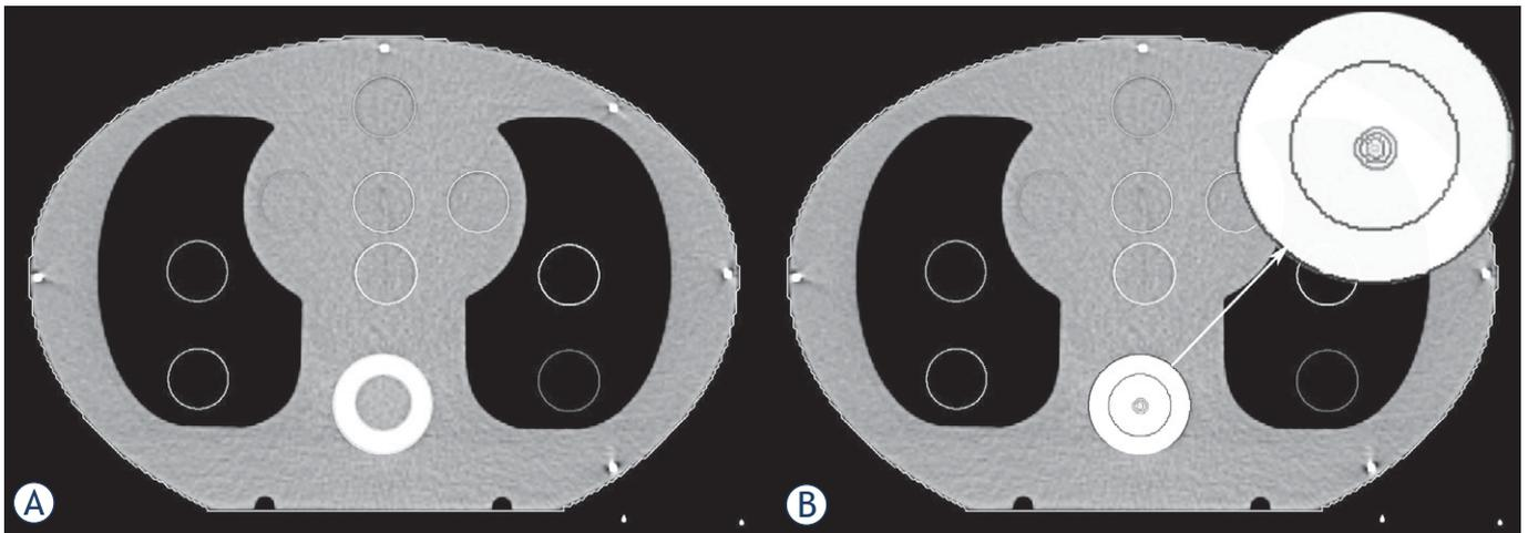
**FIGURE 2.** CT image of the CIRS Thorax phantom: water equivalent insert inside BDE part of the phantom (A); a BDE insert inside bone density equivalent (BDE) part of the phantom (B) and cross-section of small “water cylinders” of different dimensions delineated inside BDE part of the phantom to find limits for calculating geometry where cavity theory applies (top right).
