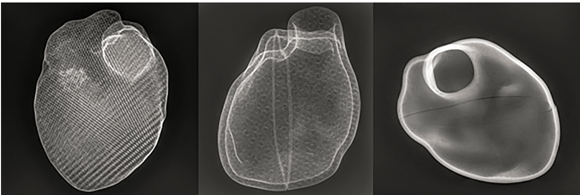
FIGURE 2. Radiographs of 3 different heart phantoms: full model with honeycomb shaped infill (A), hollow model with honeycomb shaped infill of the walls (B), and hollow model with 100% infill of the walls (C).
